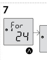
for - press  $\Delta$  to unlock the time displayformatsetting. Use  $\nabla \swarrow \nabla \nwarrow$  to scroll through the menu. Long press  $\Delta$  confirms the selection.
