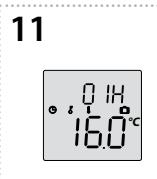
Press  $\Delta$  to unlock the temperature setting. Use the  $\nabla \swarrow \nabla \nwarrow$  shift in the temperature setting. Press  $\Delta$  to confirm the setting, while moves to the top line - set the time for holiday mode. First, the format (day / hour) is set, then the time (units, tens). Press  $\Delta$  to confirm the setting.
