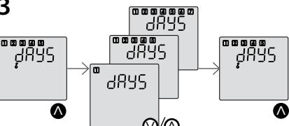
Long press of the  $\Delta$  key opens the type of time program selection - days\*. Short presses  $\nabla\Delta$  goes through the menu. Long press  $\Delta$  confirms the selection.
