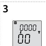
Press  $\Delta$  to unlock the RFSA-166M Compatibility Menu. Use  $\nabla \swarrow \nabla \nwarrow$  address setting. Press  $\Delta$  to confirm the setting.
