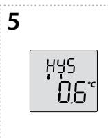
HYS - Press  $\Delta$  to unlock the heating / cooling hysteresis menu. Use  $\nabla \swarrow \nabla \nwarrow$  shift in values (range 0.2 ... 5.0 °C, step 0.2 °C). Press  $\Delta$  to confirm the setting.
